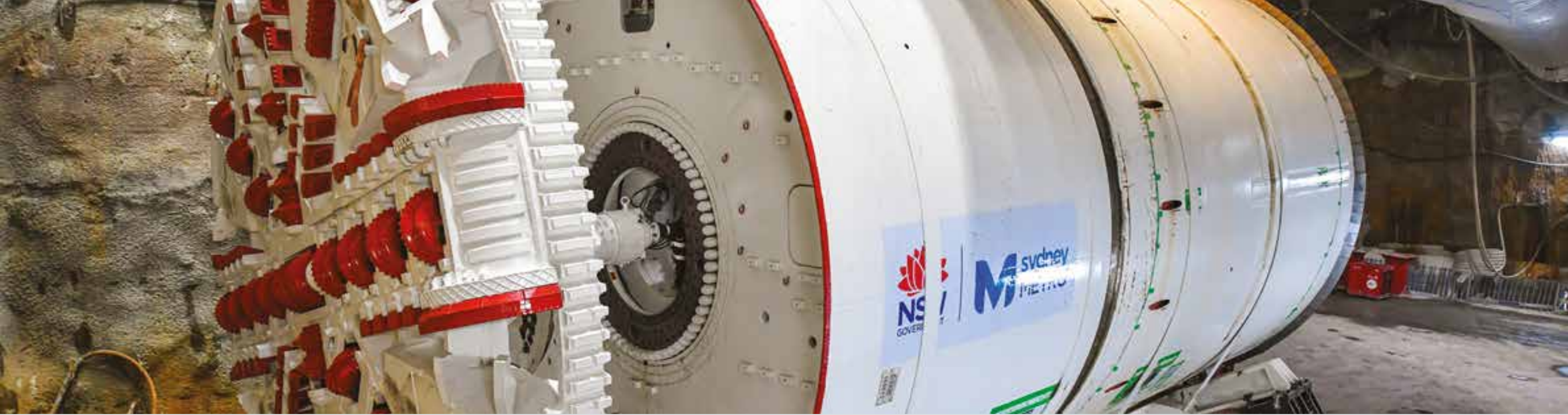
The cutterhead of TBM Kathleen used on the City & Southwest metro project.
