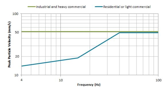
Figure 2 Transient Vibration Values for Minimal Risk of Cosmetic Damage
