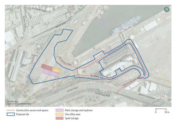
Figure 4-3: Location of construction compound and construction site access
