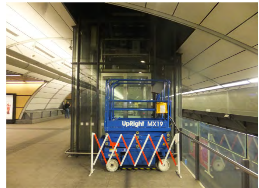
Temporary or ancillary equipment, vending machines or any other structures (i.e. temporary signage) are not be placed in the primary pedestrian paths. Source: Grimshaw.
