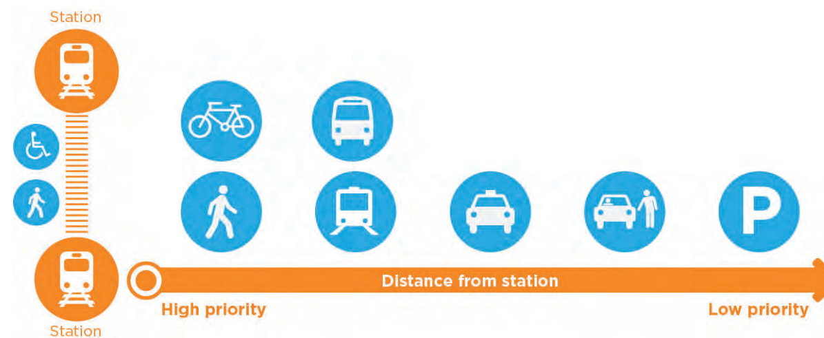
Station modal access hierarchy Source: TfNSW
