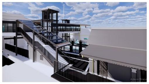
Figure 4.8 New stair, stair canopy and lift in context of heritage roof forms
