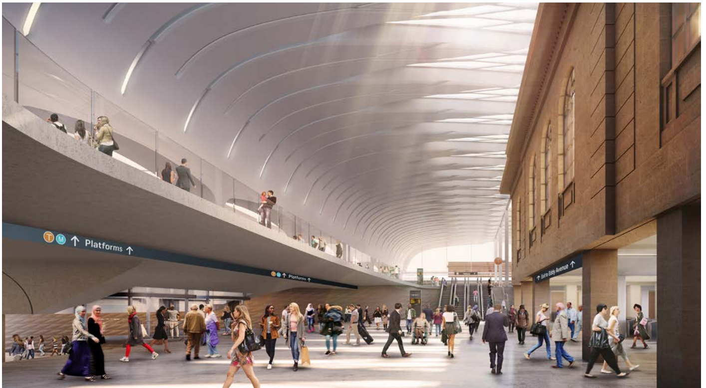
An artist's impression of the lower Northern Concourse, with the new cantilever slab on the left.
