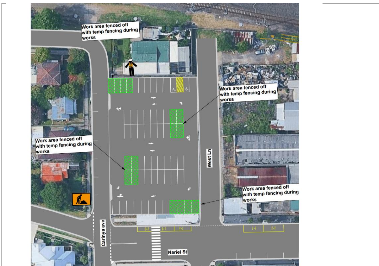
Figure 2 Geotechnical investigations locations with carspaces required to be fenced.
