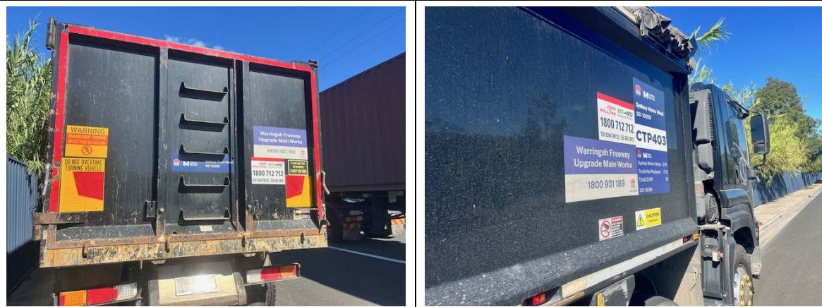
Photo 22&23: Heavy vehicle for spoil haulage not marked on the rear or sides with project details as required by Condition A46.
