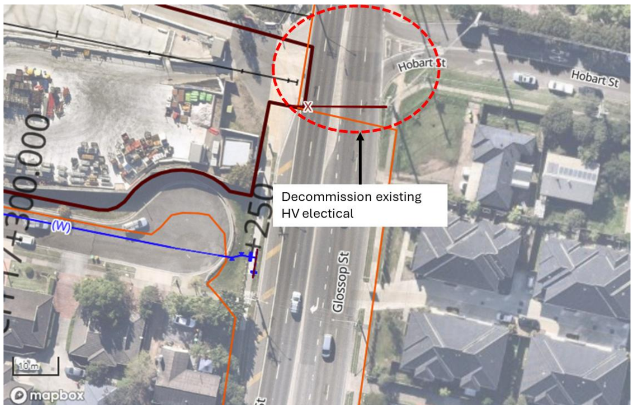
Figure 5 'Area C' Electrical decommissioning works – Glossop and Hobart Streets
