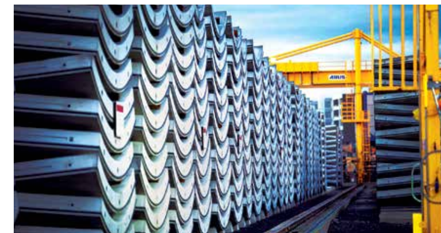
Six segments make one tunnel ring, March 2015
