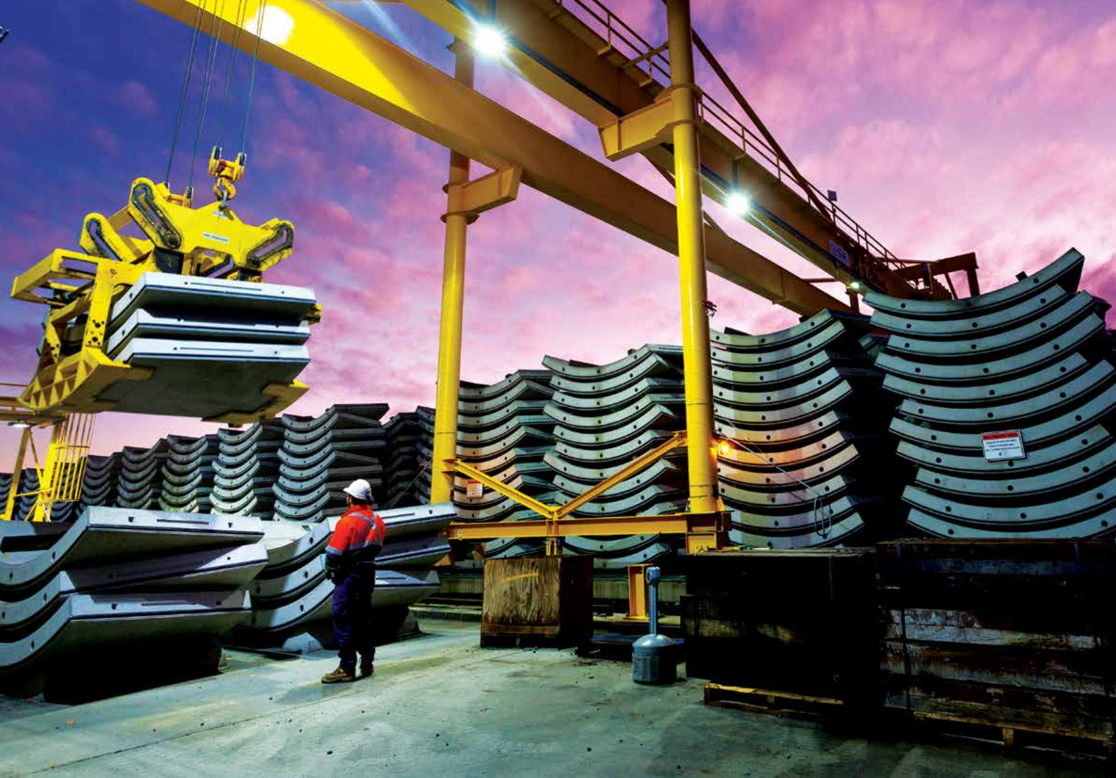
Some of the 98,184 concrete segments used to line the tunnels, Bella Vista pre-cast yard, June 2015
