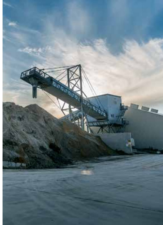
Spoil was carried by 29km of conveyor belts from the back of the TBMs to storage areas like this one at Bella Vista
