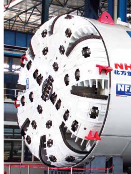
TBM1 Elizabeth factory acceptance testing, June 2014
