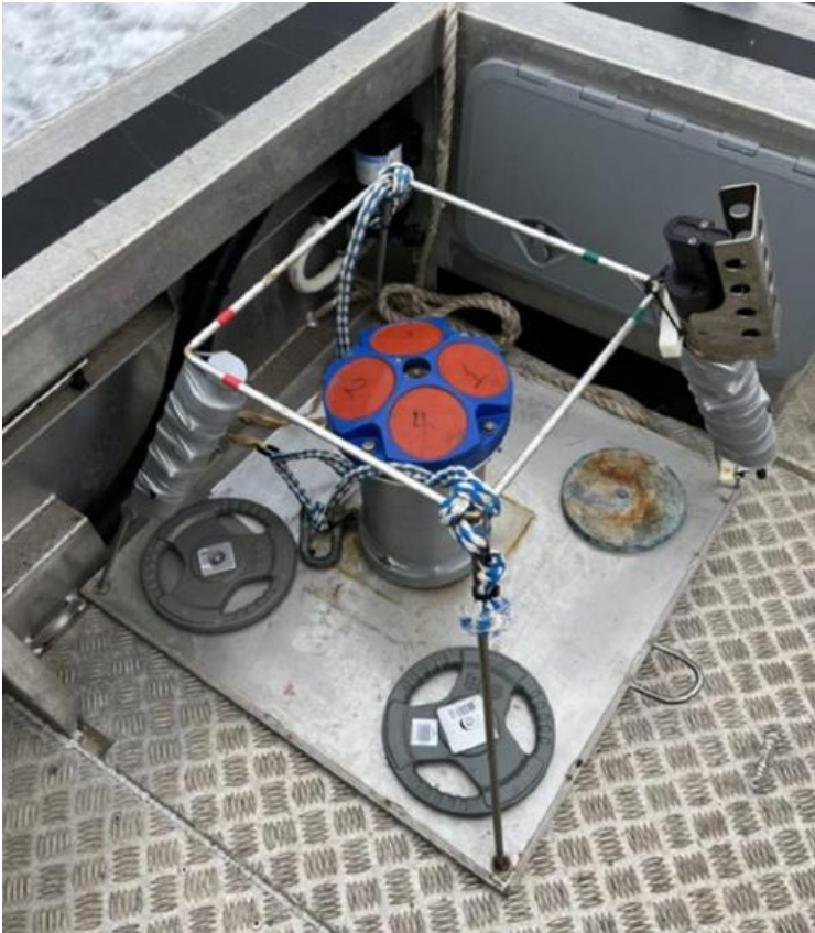
Image 2: ADCP in stainless steel frame
