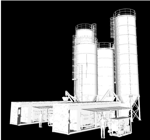
Figure 2-1 indicative drawing of grout plant
