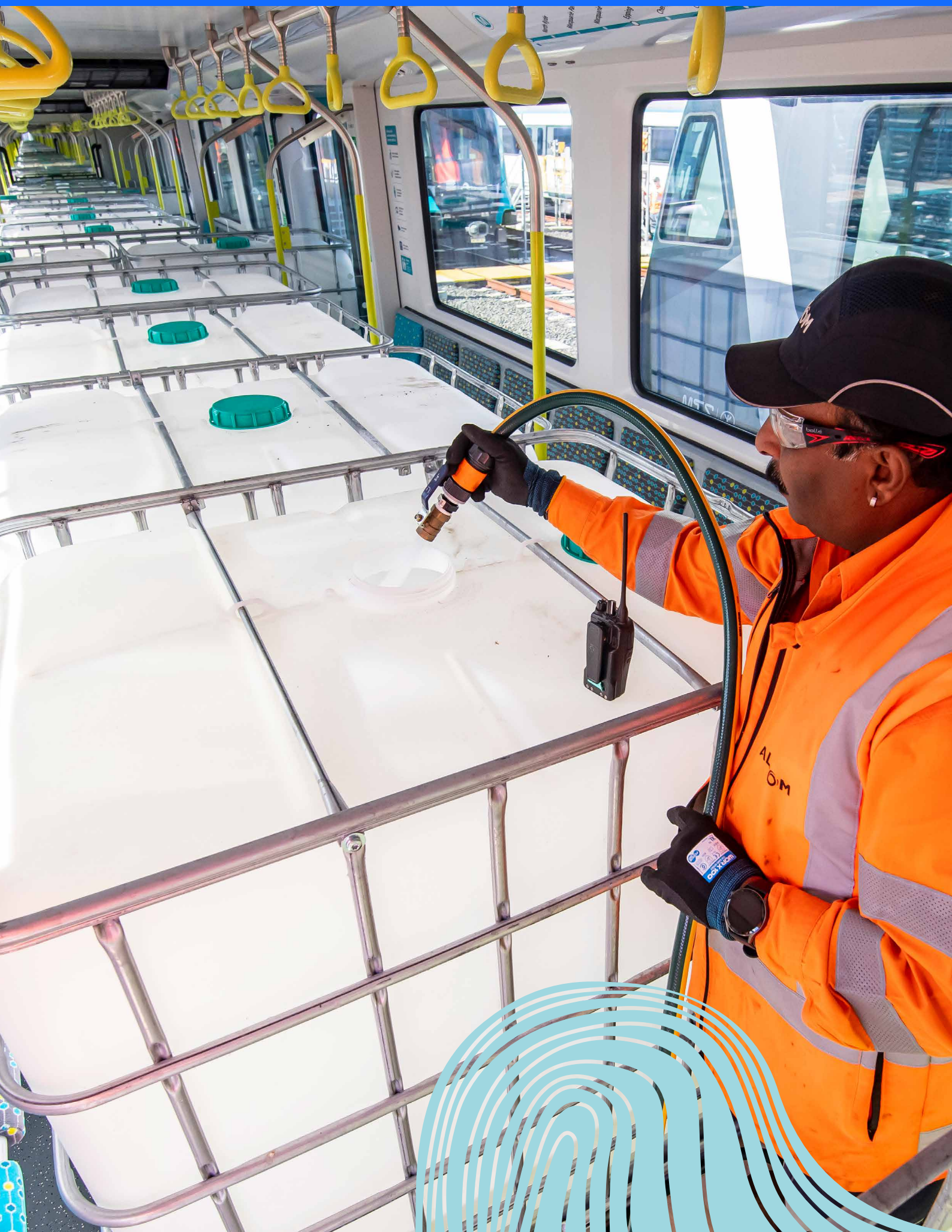
Image: During testing of the trains, full water tanks on board are used to simulate customer loads.
