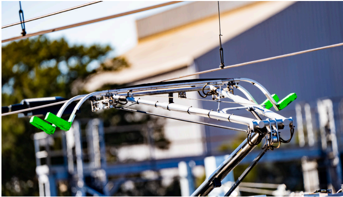
The overhead wire supplies 1500 Volts DC to the train below.
