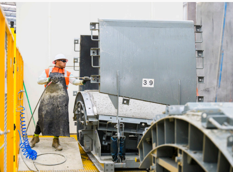
Left to right: quality checks are carried out prior to concrete pour, concrete segment leaving curing chamber and opening the mould and using scrapers to remove any excess hardened concrete.
