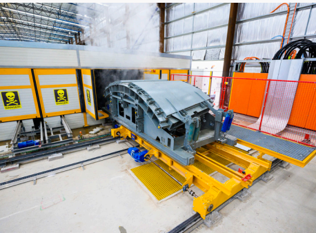
Left to right: quality checks are carried out prior to concrete pour, concrete segment leaving curing chamber and opening the mould and using scrapers to remove any excess hardened concrete.
