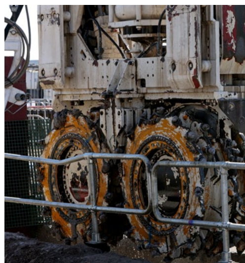
D-wall rig cutters in action
