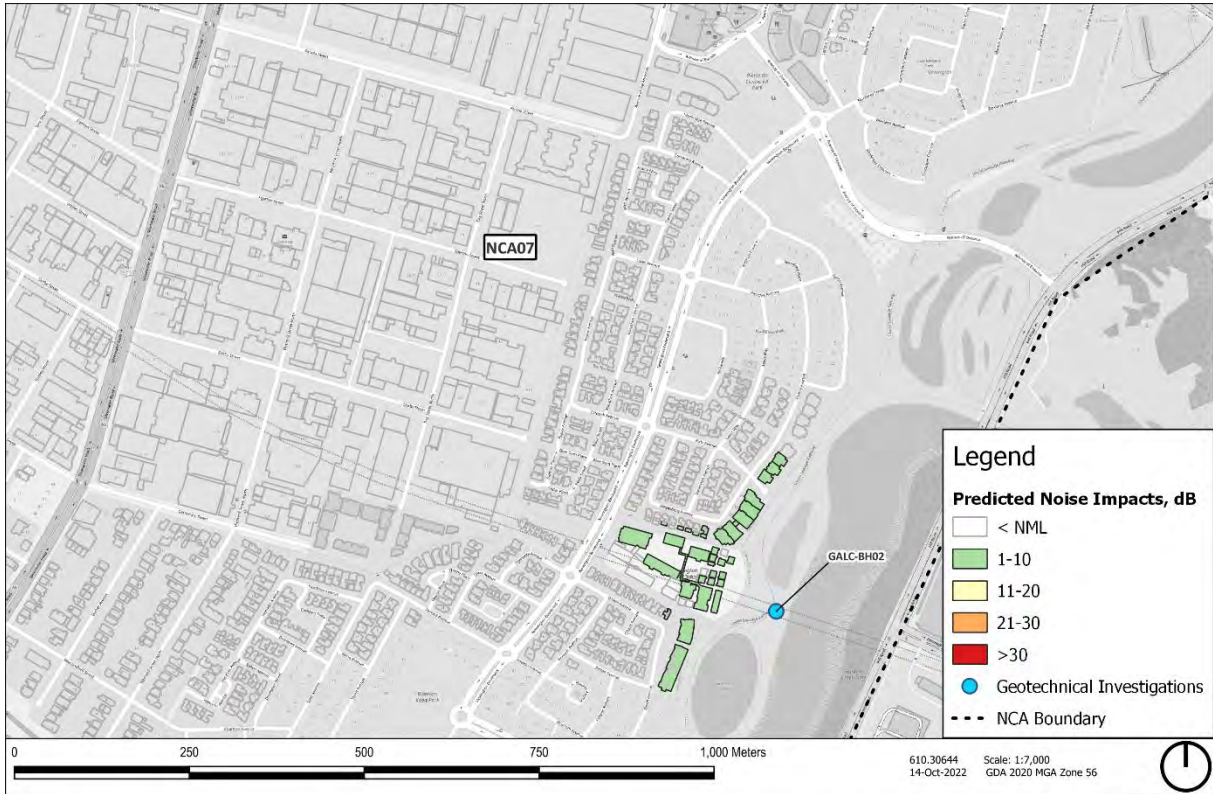
Figure A7 W.002: Drilling Operations - AH
