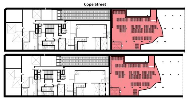
Figure 6.1.7.2: Bike hub on B1 level (below ground portion shown in pink)
