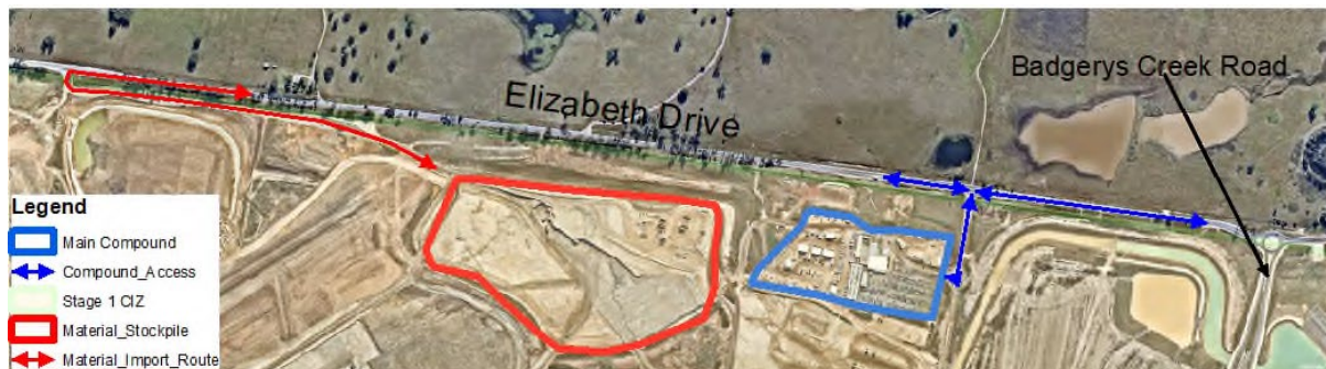
Figure 8-3 Material Importation Access arrangements
