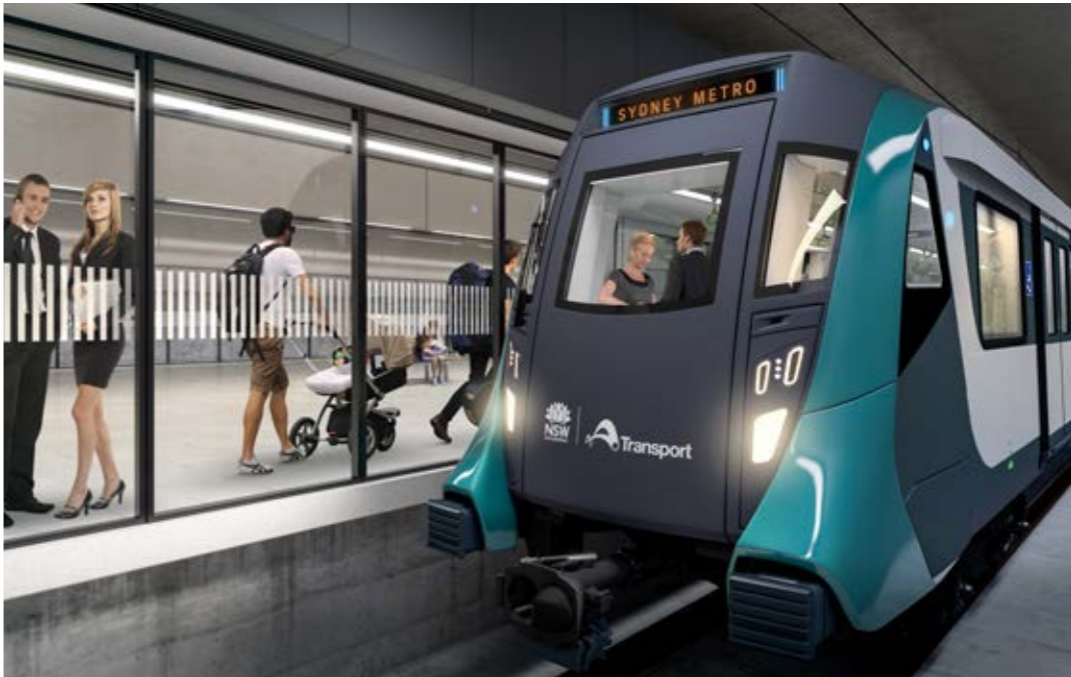
Platform screen doors keep people safe and allow trains to get in and out of stations faster.
