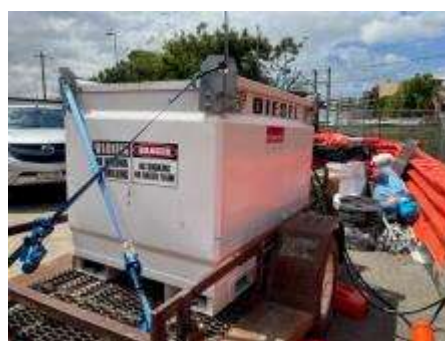
BEW North Terrace Compound: A generator and 1,000L diesel fuel cell were located adjacent to an open stormwater culvert. Controls have since been placed to reduce risk until the site compound is switched to mains power.
