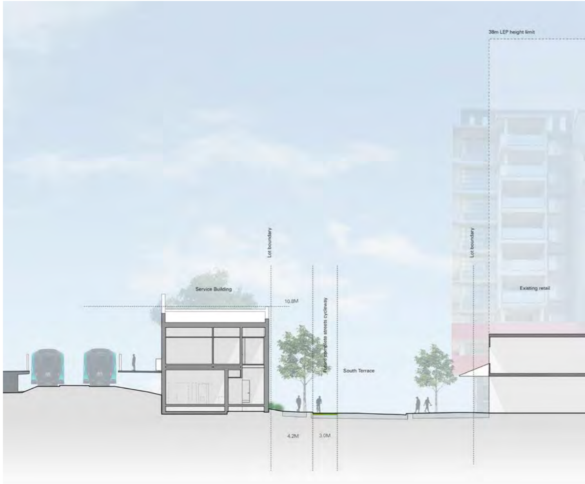
Figure 4.49 Bankstown services building section
