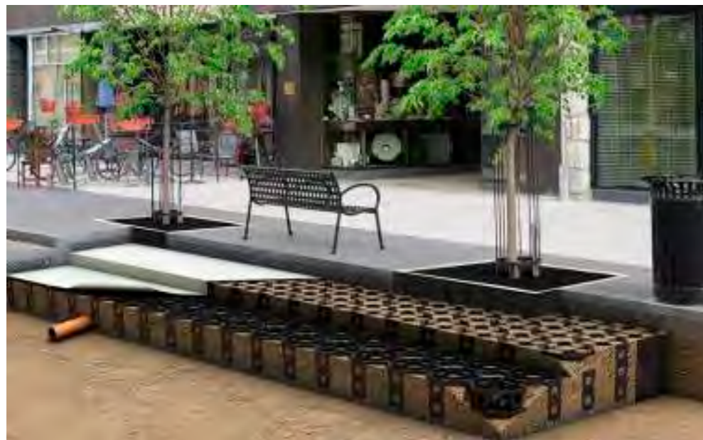
Figure 4.39 Water sensitive Urban Design soil cell system
