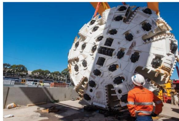
A TBM cutterhead
