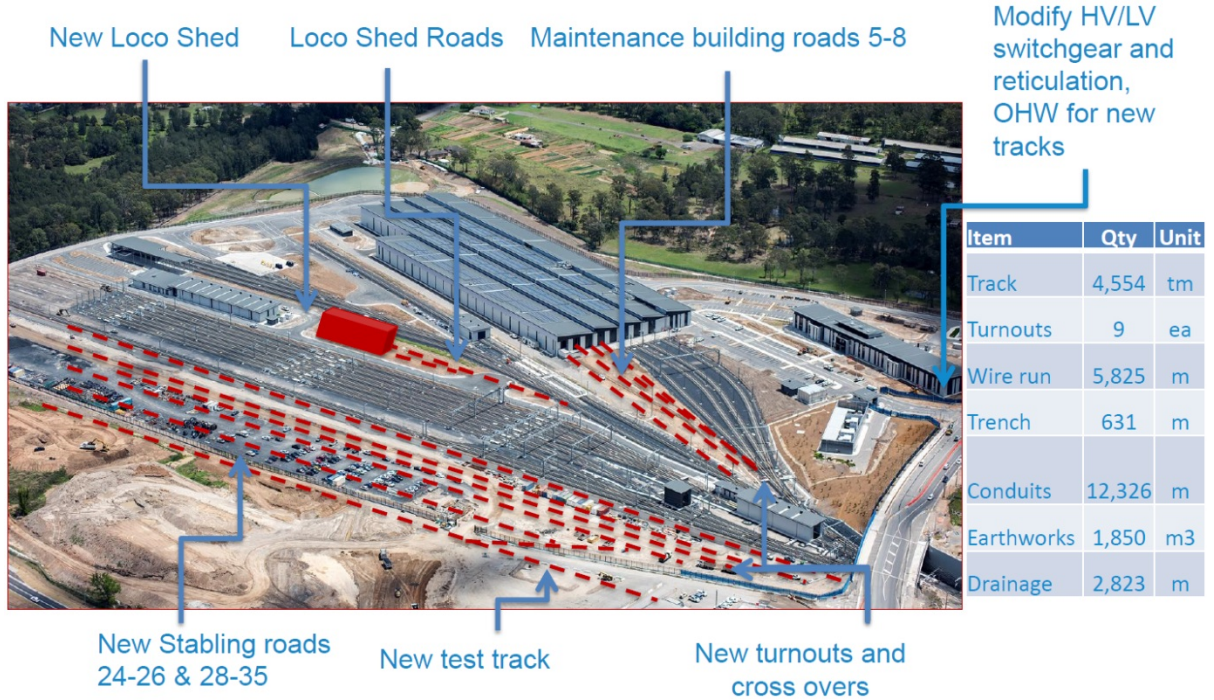
Figure 2: Indicative LW Stage Scope of Works
