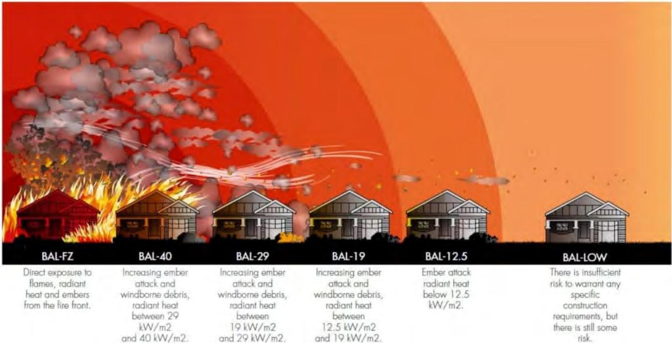
The BAL assessment (Figure 8) has been completed based on the current site boundary and the assumption that all vegetation (if any) within the proposal site would be managed as an APZ. This is with the exception of the environmental protection area which would be retained.
