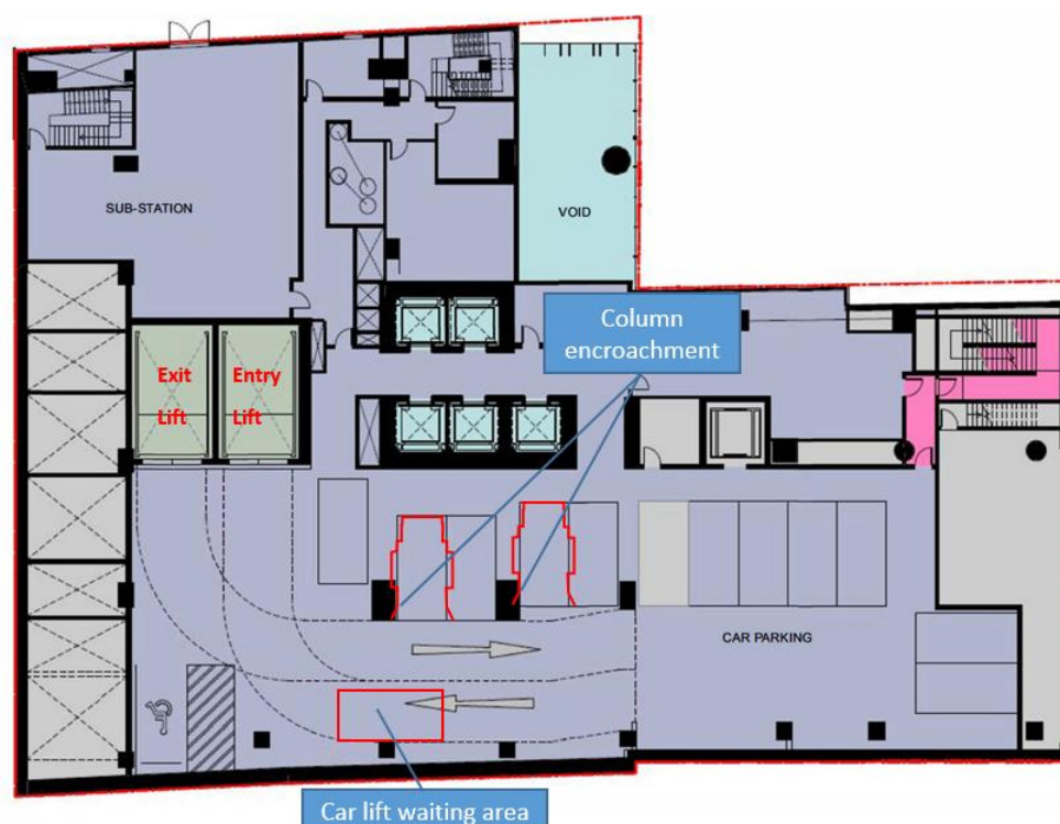
Figure 18 Car space design envelope and car lift waiting area
