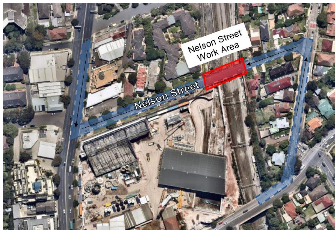
Figure 5 – Nelson Street Access and Haulage Routes
