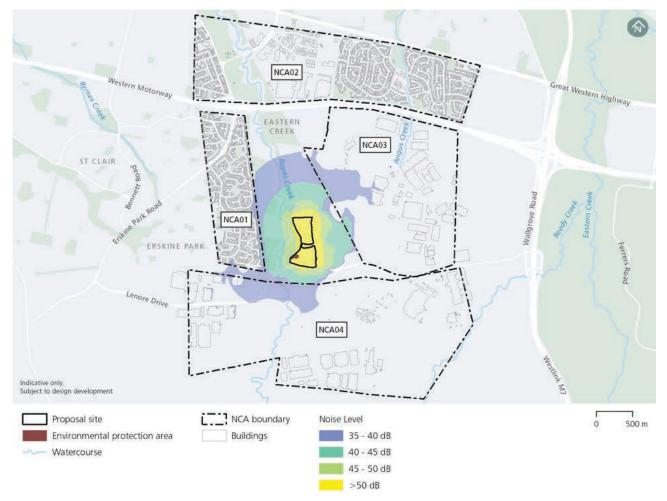
Figure 8-3: Predicted operation noise level contours
