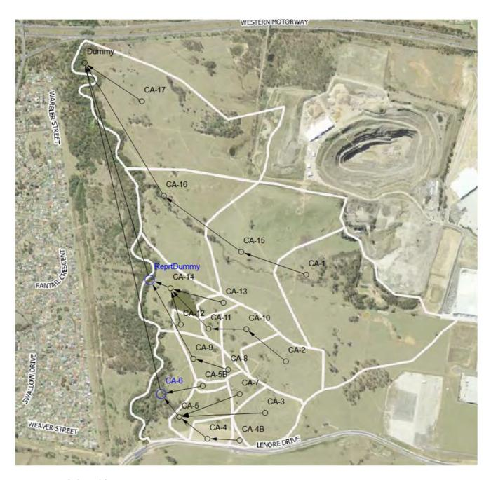
Figure A-2: XP-RAFTS layout – Existing case
