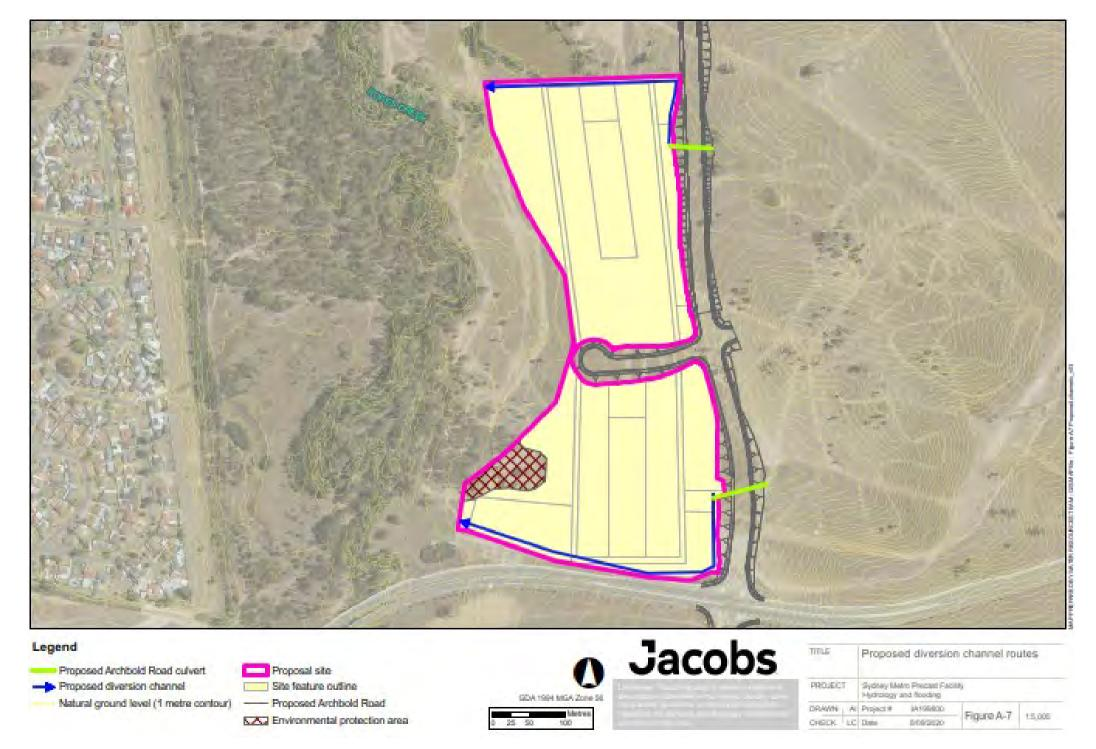
Figure A-7: Proposed route of external flow diversion structures
