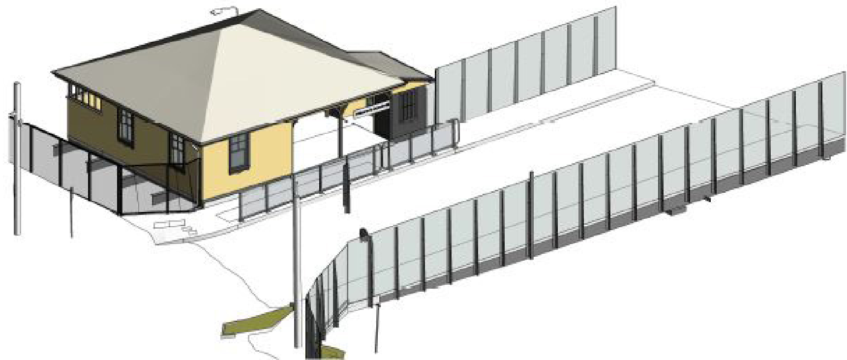
Figure 4.32 Throw screen arrangement at Wardell Road overbridge
