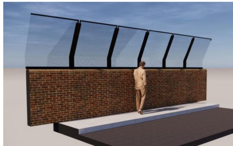
Figure 4.23 Typical Type 1 vertical protection screens
