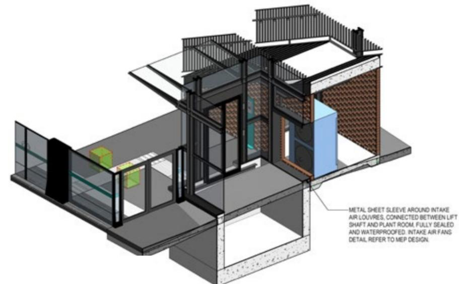
Figure 4.14 Relationship of lift with understair service zone
