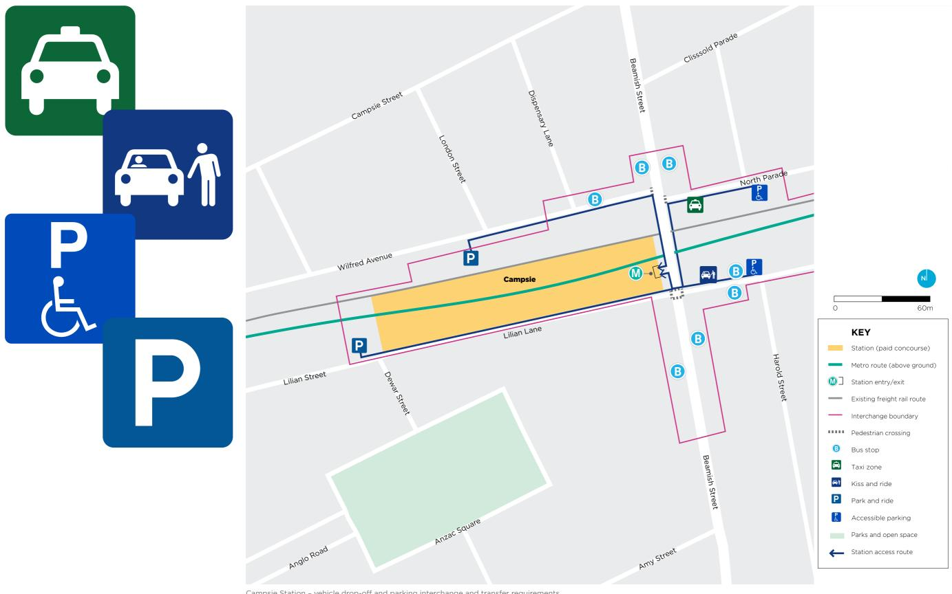
Campsie Station - vehicle drop-off and parking interchange and transfer requirements
