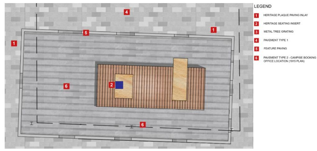
Figure 4.13 Paving inlay and seat element detailed plan
