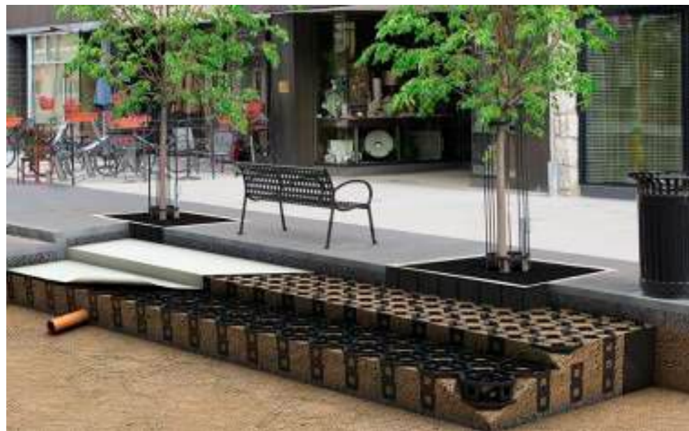
Figure 4.39 Water sensitive Urban Design soil cell system
