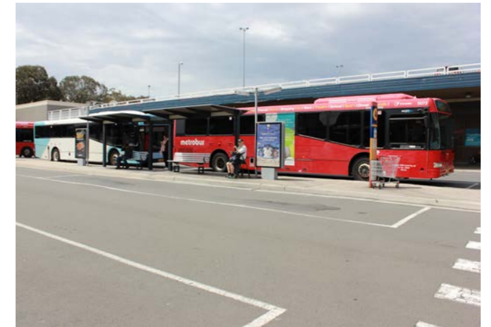
Centro Interchange: Poor Placement of seating results in Functionally Narrow Footpaths
