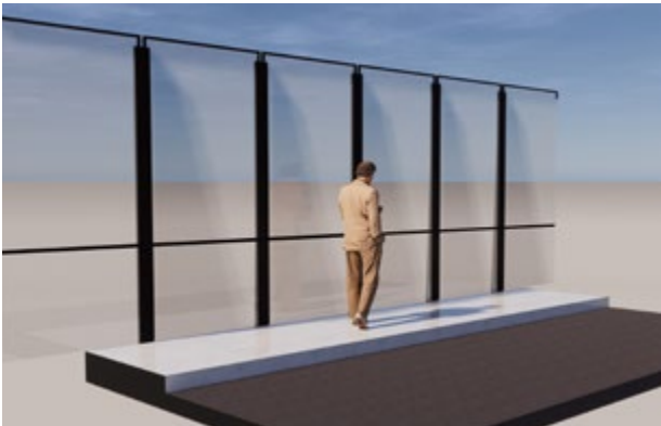
Figure 4.25 Typical Type 2 vertical protection screens
