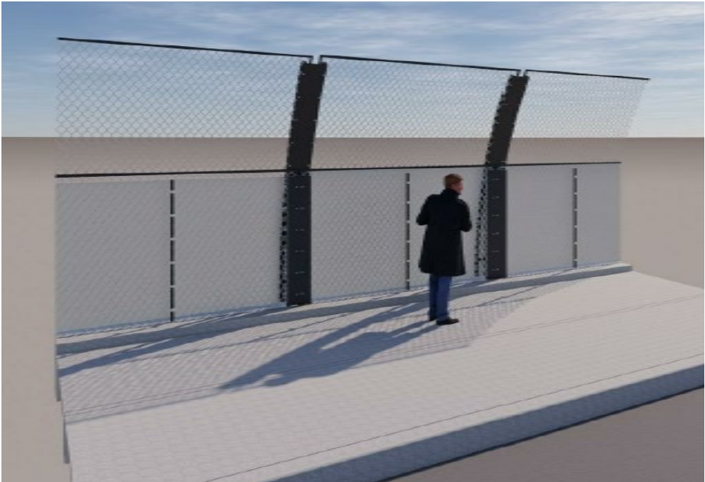
Figure 4.30 Typical Type 3B vertical protection screens
