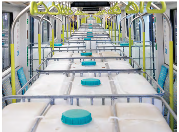
The loaded testing train has been loaded with 106 large containers filled with a total of 115,500 litres of water – the equivalent of 1540 passengers.
