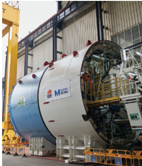
Tunnel boring machine being Factory Acceptance Tested.
