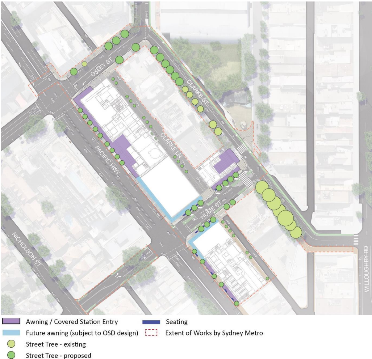
Figure 4-2 Pedestrian amenity including shade trees, covered footpaths and seating
