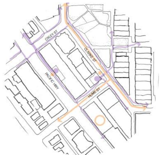
Figure 4-6 Local pedestrian (purple) and cycle (orange) connections are integrated into the design
