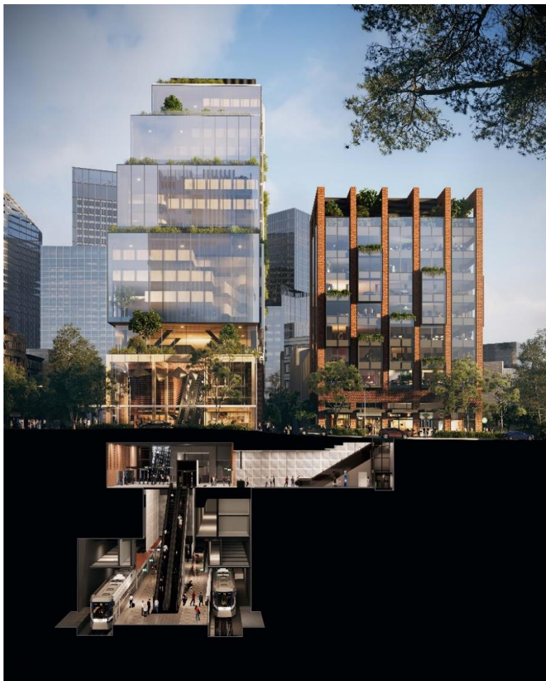
Figure 6-5 4 Hume Street elevation showing below ground station (Site A & C built form)
