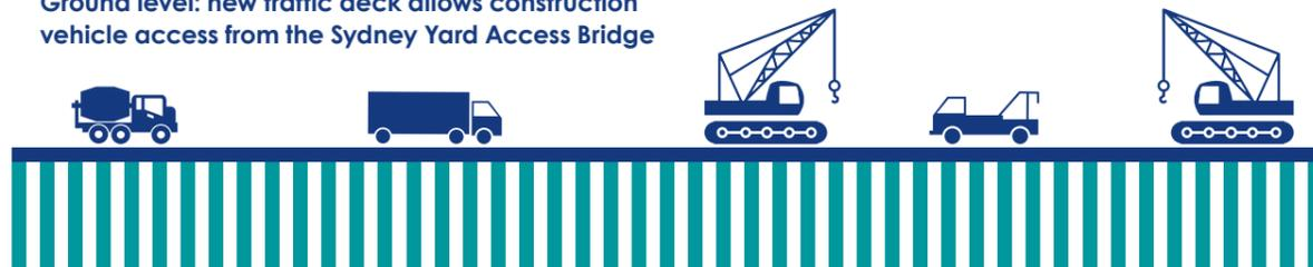
Excavation: piling and construction for the new underground metro happens underneath the traffic deck
