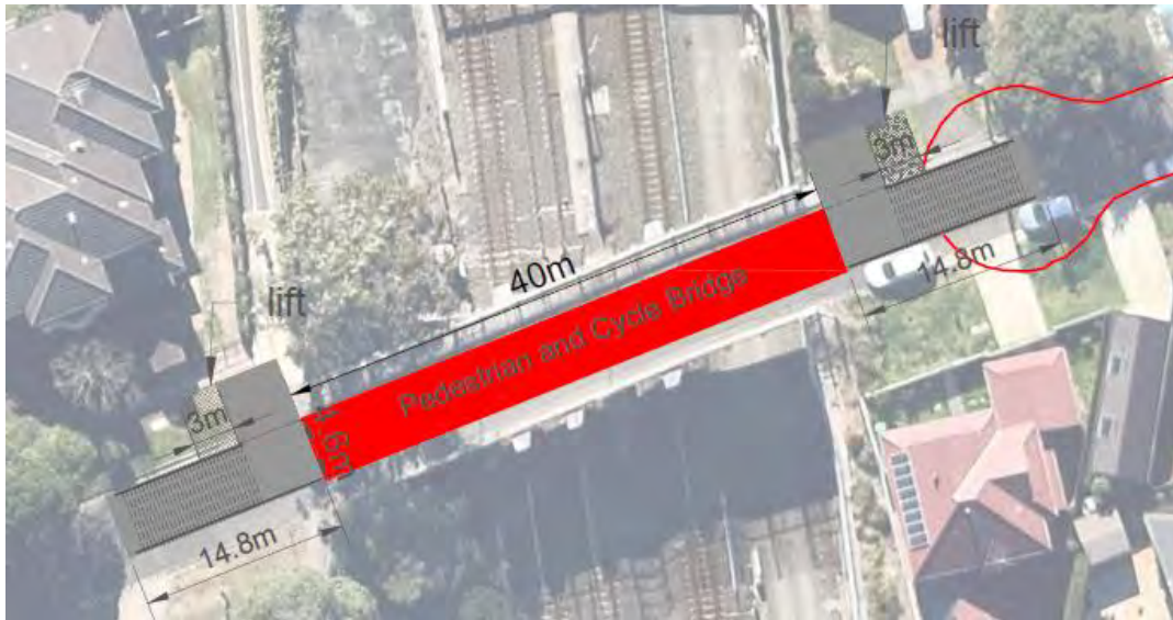
Figure 27: Nelson Street Stairs and Lift option – footprint
