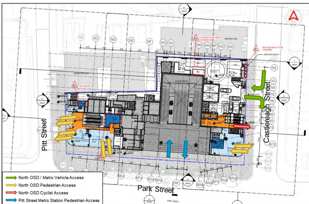
Figure 2-1: North OSD access locations on the ground floor (Reference: SMCSWSPS-FOS-OSN-AT-DWG-030013 Rev P1)
