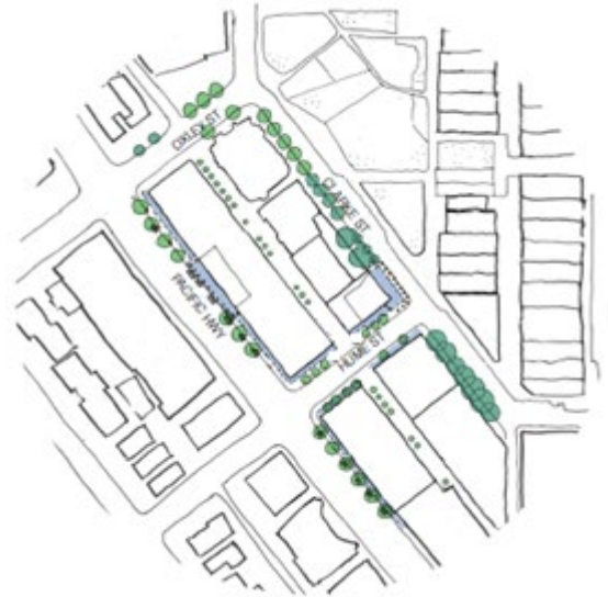
Figure 4-5 Street trees, awnings and seating provide a comfortable and safe pedestrian environment
