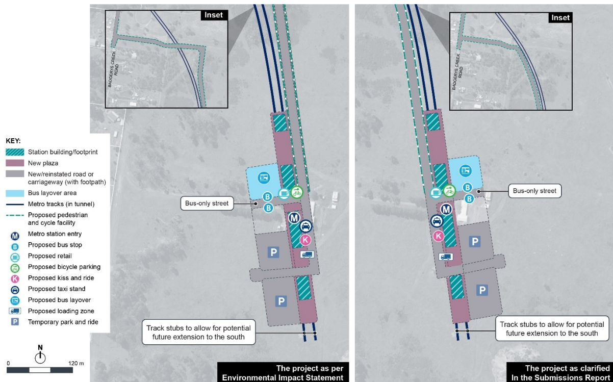
Figure 6-6 Aerotropolis Core Station - Indicative layout and key design elements Note: Indicative only, subject to design development.
